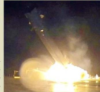
Attempt to land a Falcon 9 booster on Jan. 10, 2015, ended in a crash after the booster ran out of hydraulic fluid for the steering fins.
