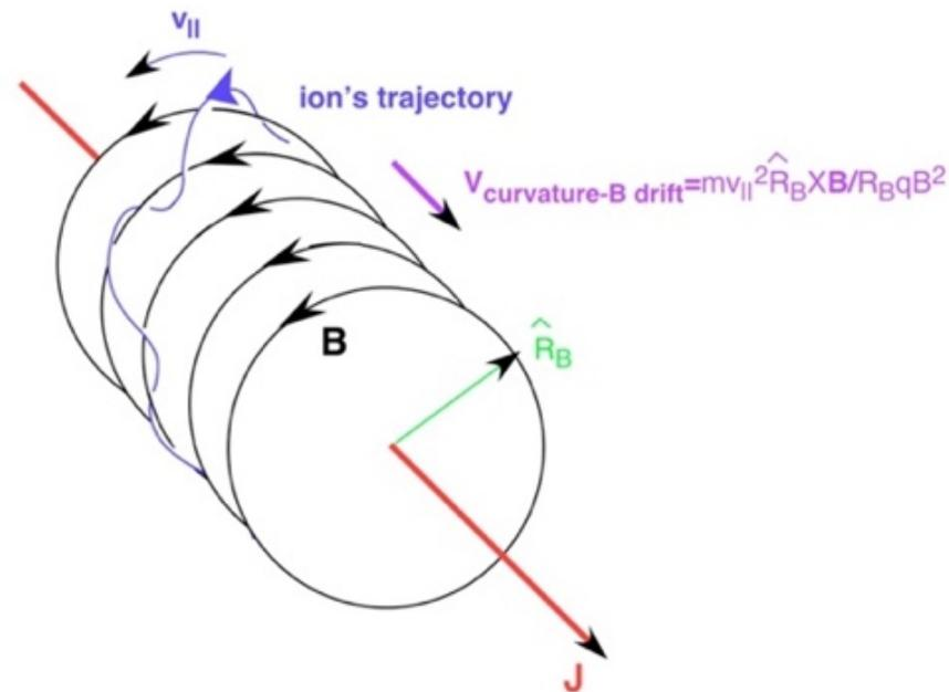
Fig. 5.3. A sketch of curvature drift of an ion.
