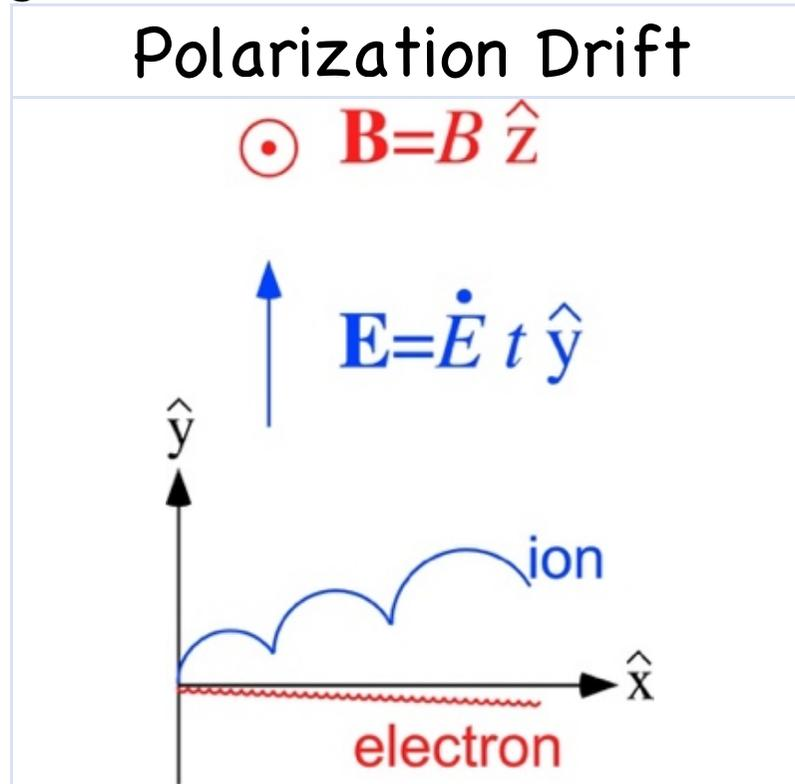
Fig. 5.2. A sketch of polarization drifts of an ion and an electron.
