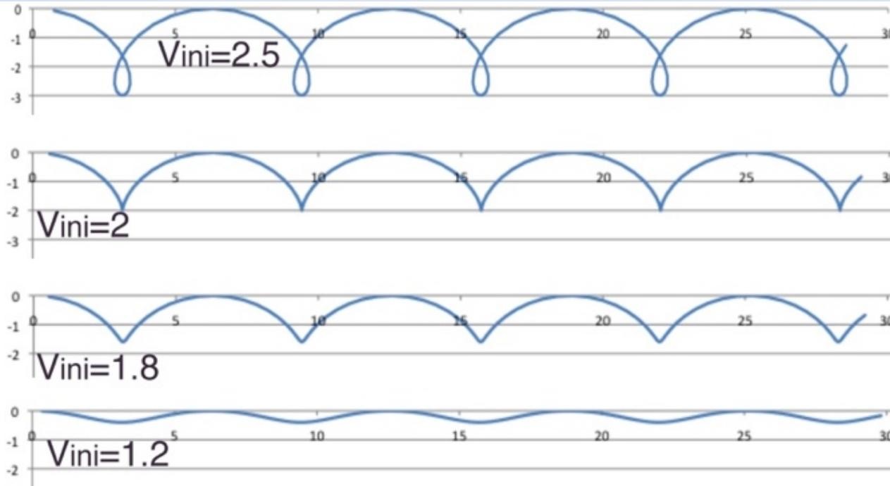
Fig. 5.1. Examples of  $E \times B$  Drift
