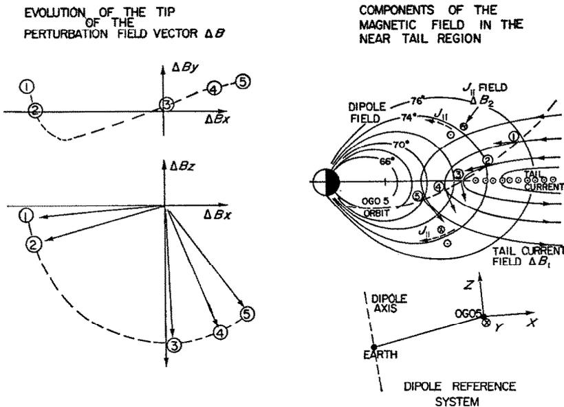
FIG. 2. SCHEMATIC FIGURE SHOWING IN UPPER RIGHT PANEL THE THREE MAIN SOURCES OF MAGNETIC FIELD IN THE NEAR TAIL REGION, EARTH'S DIPOLE, FRINGING FIELD OF THE TAIL LOBES AND FIELD ALIGNED CURRENTS.
