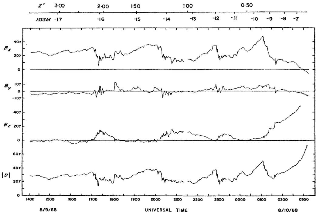
FIG. 6. UCLA FLUXGATE MAGNETOMETER OBSERVATIONS ON OGO 5 ON AUGUST 9-10, 1968. Four successive substorms cause systematic changes in the field components in relation to expansion onset. As shown in two following figures onsets are nearly at the times of peak field magnitude.
