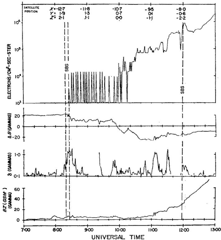
FIG. 3. TYPICAL INBOUND PASS OF OGO 5 ALONG TRAJECTORY SIMILAR TO THAT OF FIG. 2. Data include from top to bottom flux of energetic electrons ( $E \geq 50$  keV), deviation of observed field magnitude from dipole magnitude, rms amplitude of magnetic field fluctuations of frequency greater than 0.07 Hz, and the Z-component of the field in GSM coordinates. Vertical dashed lines are the onset times of substorm expansions determined from midlatitude ground magnetograms.
