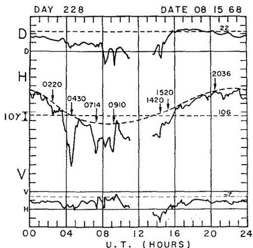
FIG. 13. MAGNETIC FIELD OBSERVATIONS AT SYNCHRONOUS ORBIT (150°W LONGITUDE) MADE BY UCLA FLUXGATE MAGNETOMETER ON ATS 1.
